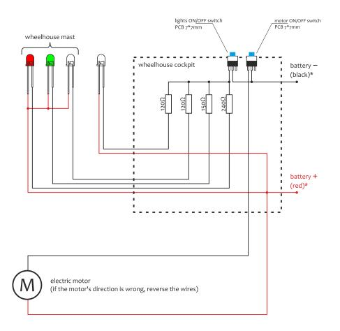
\* you can use male/female jumper wires to easy and fast connect/disconnect battery and wheelhouse module
